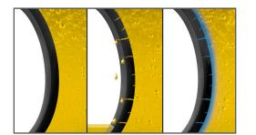
Performance Plus<sup>®</sup> Synthetic Blend High Mileage Passenger Car Motor Oils are blended with a special additive package designed for older vehicles or those with high miles. These additives cause a chemical reaction with the elastomeric seals and gaskets to cause a slight swell to improve protection and aid in the sealing of leaks all the while continuing to provide sludge and deposit control.
